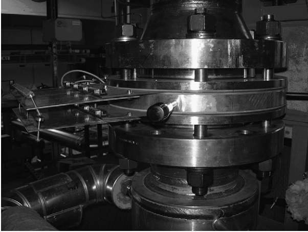
Fig. 3. The installed wire-mesh sensor with two measuring planes.
